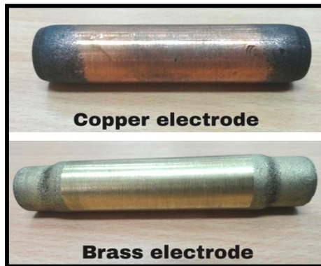
Figure (3) copper and brass electrode after machining.
