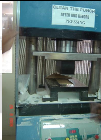
Fig.2: Samples preparation by Hydraulic Press
