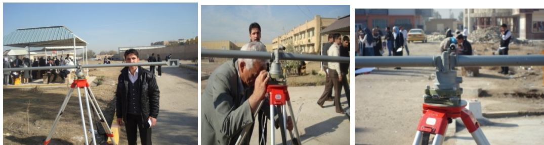
Figurer 8 Measuring distance by subtense Bar
