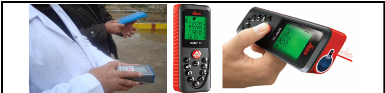
Figure 7 measuring a distance by disto-light (D5)
