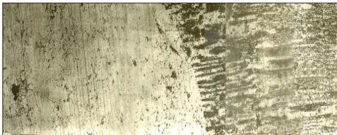
Figure (4) Weld joint of Plasma welding
