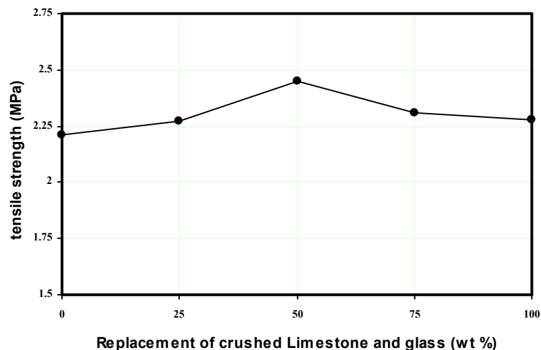
Figure (3): Mortar Tensile strength with Replacement ratios of crushed limestone and glass.
