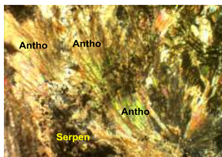
Fig.(14): the amphibole (anthophyllite) after pyroxene due to uralitization (XN)-(40X)
