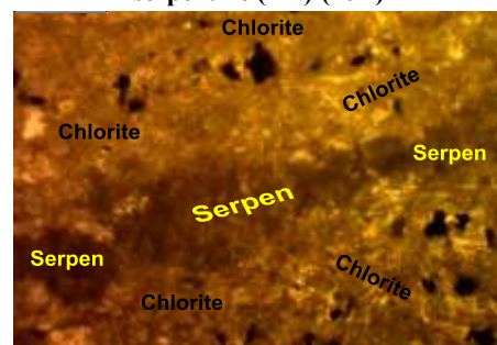
Fig.(17): Chlorite after pyroxene cut with serpentine (XN)(40X) .
