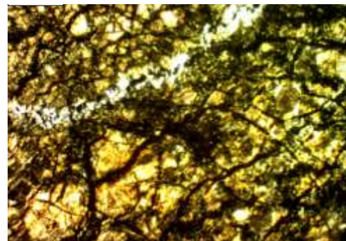
Fig (3b): Mesh texture in olivine crystals in fine background of serpentine. It is named hourglass texture (PPL)-(40X) .
