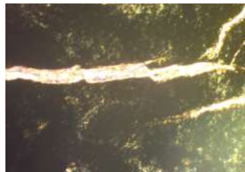
Fig.(4): Fibrous texture which appears a mixed background of talc and serpentine minerals cut by granules of magnetite that spread randomly within background (PPL)-(40X) .
