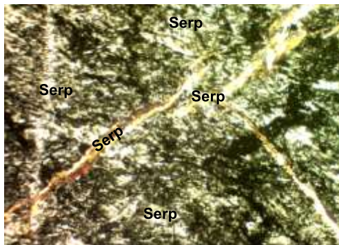
Fig.(5): Fibrous interlocking texture as rectangular canals of serpentine cut by veins of secondary serpentinite (PPL)-(40X) .
