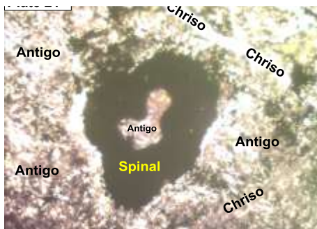
Fig.(20): Zoning of spinel mineral in a background of serpentine (PPL)-(40X)
