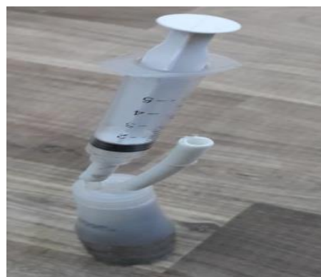
Figure 3.Hydrogen gas dryingand storage system
