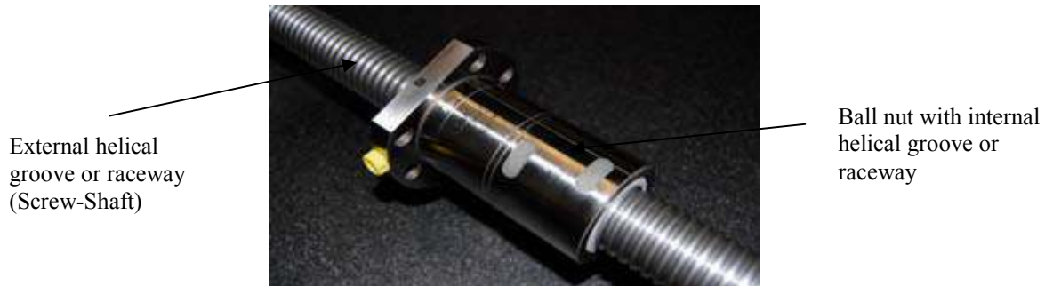
Figure (1) Ball-Screw-Assembly (BSA)
