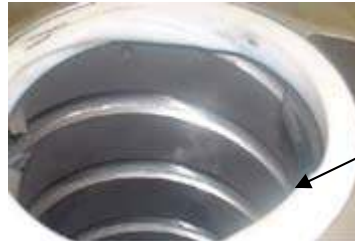
Figure (2) The effect of fatigue on ball nut surface
