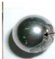
Figure (3) The effect of adhesive wear on Ball surface
