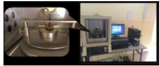
Figure (3) Thermal conductivity measuring device.
