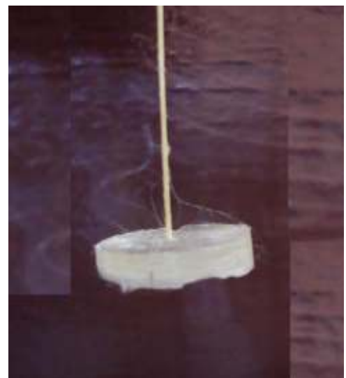
Figure ( 5): Pull out test specimens preparation assembly
