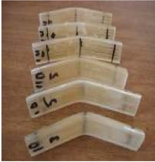
Figure (8): Failed bending specimens Figure ( 9): Relation between the bending stress and the fiber density
