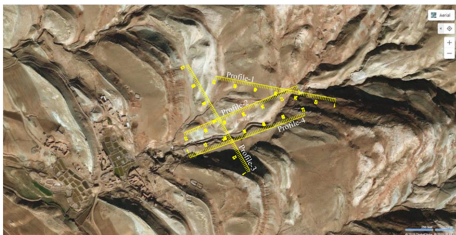
Fig. 5 Satellite image showing the geoelectric survey profile
