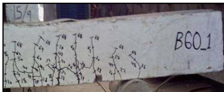
Figure (4.5) Crack pattern for strengthened beam B60-1
