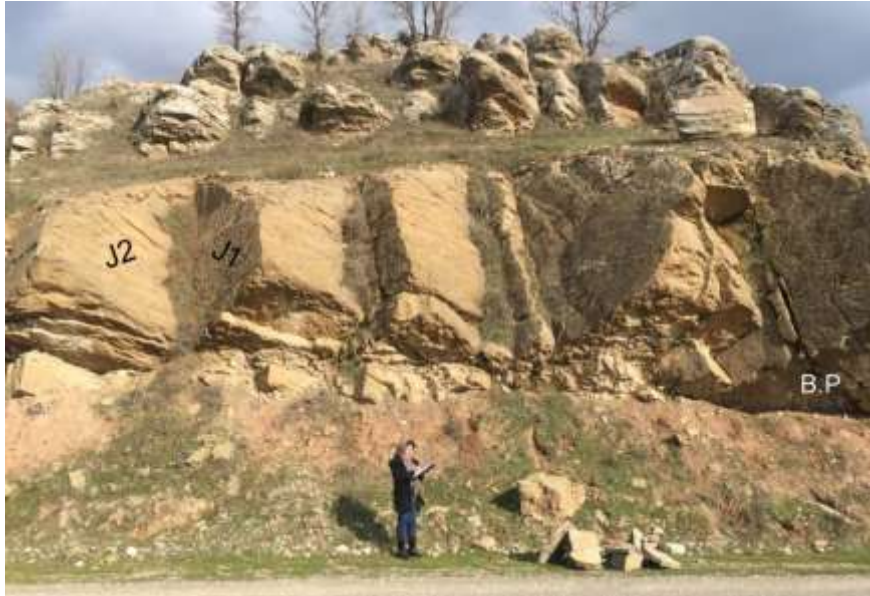
Fig. 10: General view for slope at station no.3 with marked discontinuity sets
