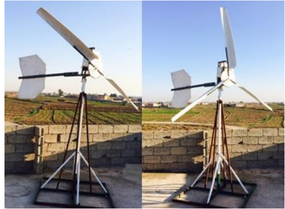
Fig 1: Homemade wind turbine when use two and three blades
