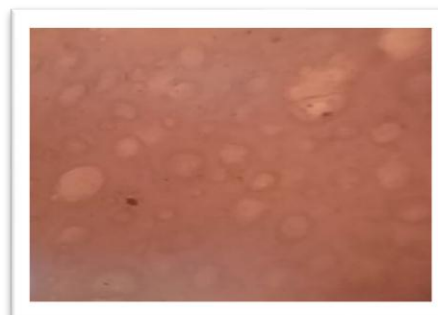
Fig. 3: Microscopic examination of a section of a thermally treatment sample for a period of (6 hours) and with a treatment temperature ( T=70^{\circ}\text{C} ). It shows almost no defects. (x400).
