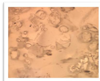
Fig. 9: Microscopic examination of a section of the friction surface that is subject to heat treatment for a period of (6hur) and with a treatment temperature of ( T=70^{\circ}\text{C} ). (x400)
