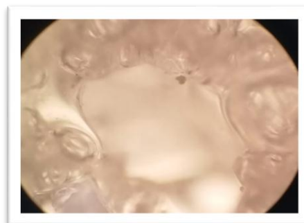
Fig. 8: Microscopic examination of a section of the friction surface that is not subject to heat treatment. (x400)
