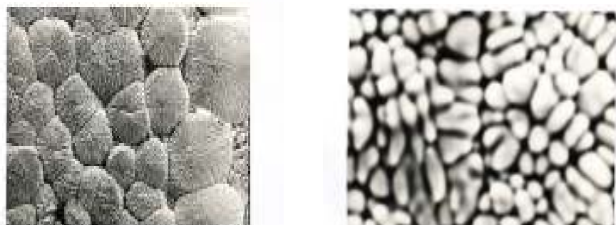
Fig. 3: Higher magnifications of the plan view of sealed layer showing the cells.
