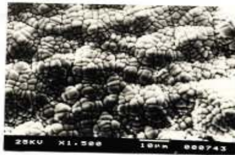
Fig. 6: Higher magnifications SEM photograph showing the cells inside the porosity.
