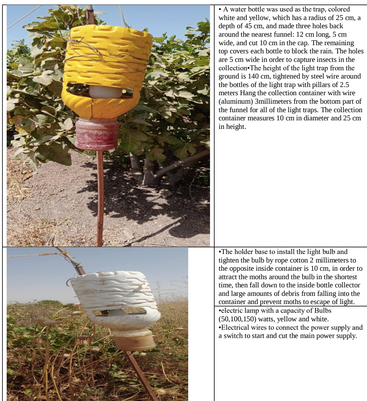
Figure 1; A- The local design of a light traps and its specifications
