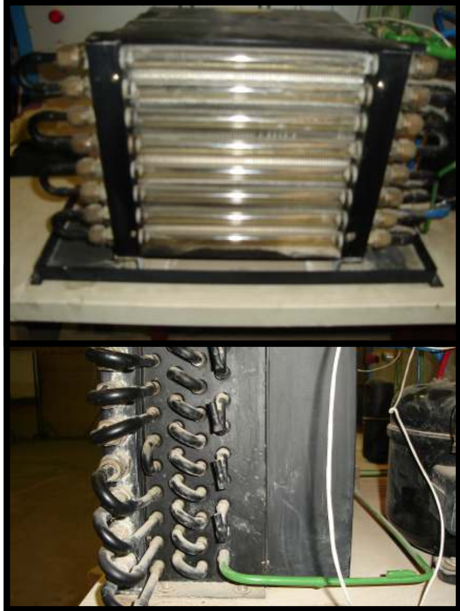
Fig.1. The condenser of the unit under
