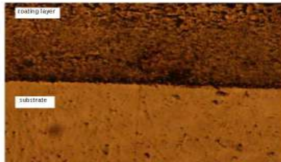
Fig (11) 5hr Aluminide Coating at 1000 °C, 50 hrs Heat Treatment at 1000 °C for AISI330 St.St. Specimens
