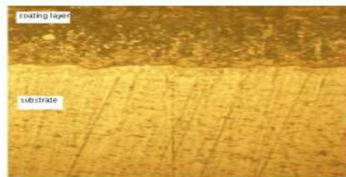
Fig (7) 3hr Aluminide Coating at 1000 °C, 5 hrs Heat Treatment at 1000 °C for St.St AISI330 Specimens at x150
