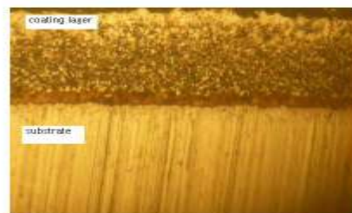
Fig (9) 7hr Aluminide Coating at 1000 °C, 5 hrs Heat Treatment at 1000 °C for St.St AISI330 Specimens at x150
