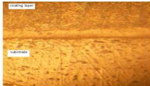
Fig (4) 5hrs Aluminide Coating at 1000 °C for St.St AISI330 Specimens at x400
