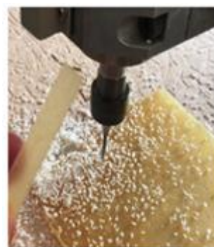
Fig. 1: Rotary head of (CNC) machine and specimens cutting by (CNC) machine.
