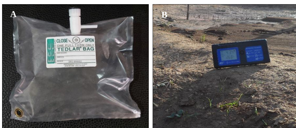
Fig. 6: A) Tedlar Bags ESS for gas composition analysis B) \text{CO}_2 meter Air \text{CO}_2 ntrol 3000
