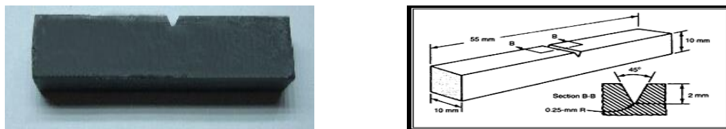
Figure 1: The shape and dimensions of the sample prepared for the shock resistance test
