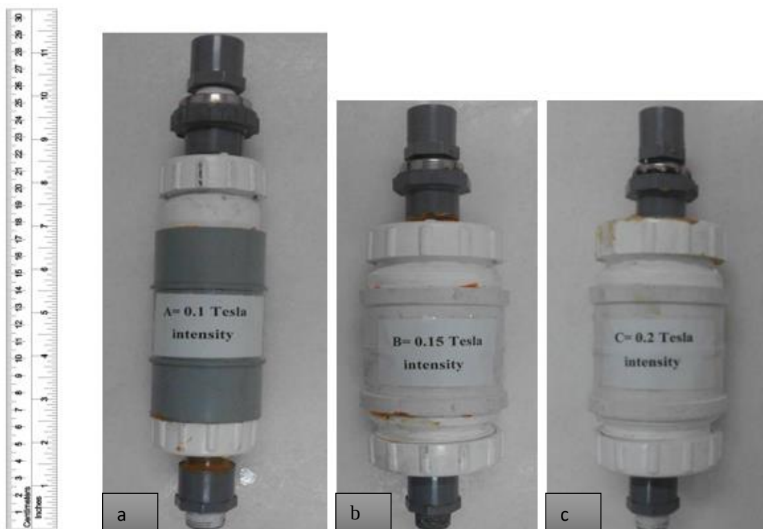
Figure 1 The magnetic devices of different intensities used in the experiment (a) 0.10 T (b) 0.15 T(c) 0.20 T.
