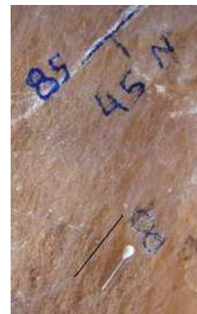
Fig. 11. Part of the top surface of sample No 2 which contains striations that make 15^{\circ} E as pitch angle with the strike line of the vein( pin length is 1cm, the pin is parallel to striation ).
