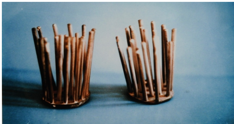
Figure 1: Photograph of the cast rods oriented over crucible former after casting.
