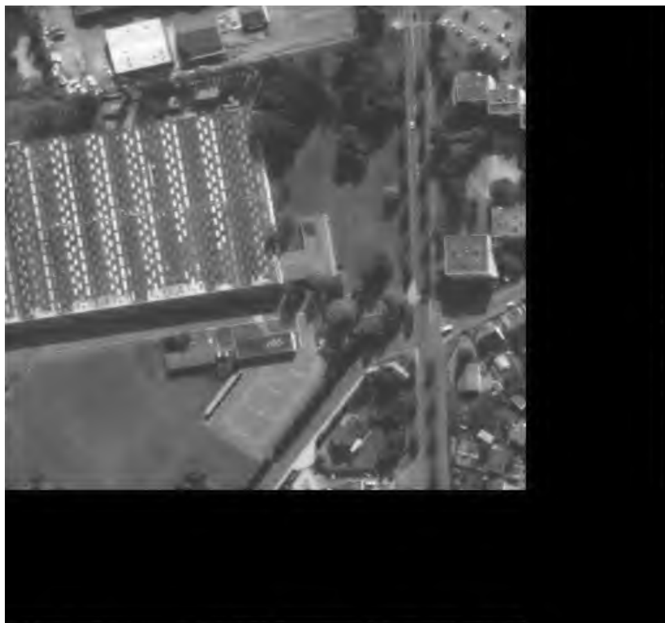
Fig. 5 The reconstructed image «Town» fragment 400×400 using the compression coefficient equal to 16, the adaptive wavelet transform and the biorthogonal wavelet 9.7
