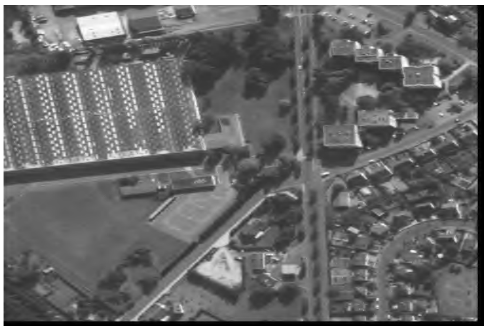
Fig. 6 The reconstructed image «Town» fragment 500×500 using the compression coefficient equal to 16, the adaptive wavelet transform and the biorthogonal wavelet 9.7
