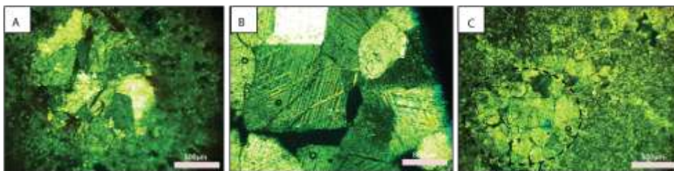
Fig. 6: The Cement types from different parts of Pila Spi Formation from Sarkand and Gulley Keer sections. (A) Granular cement from the lower part of formation from Sarkand section P.P.L (4X), SA.6, B.R. (B) Blocky cement filled the molds of previously dissolved skeletal grains from the upper part of Pila Spi Formation from Sarkand section P.P.L (4X), SA.23, B.R. (C) The drusy cement in the lower part of Pila Spi Formation from Gulley Keer section P.P.L (4X), GK.5, B.R
