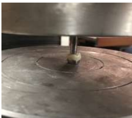
Figure (3): Acrylic PMMA sample under universal testing machine for fracture testing
