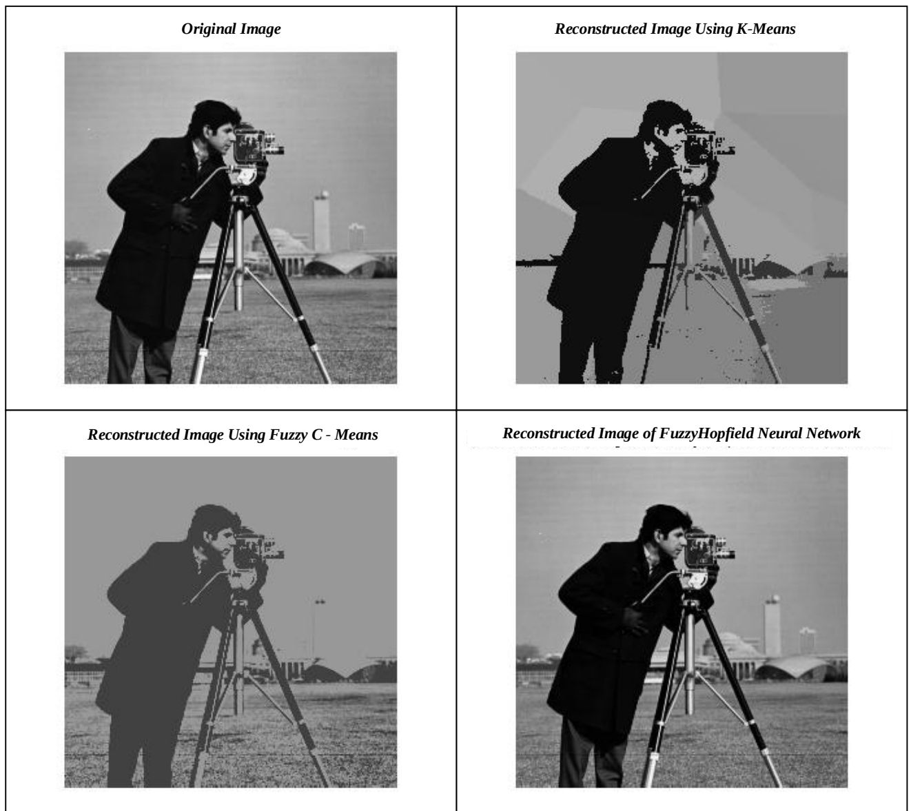
Fig. 7 : Original image , Reconstructed image using K-means, Reconstructed image using fuzzy c-means, Reconstructed image using fuzzy Hopfield neural network
