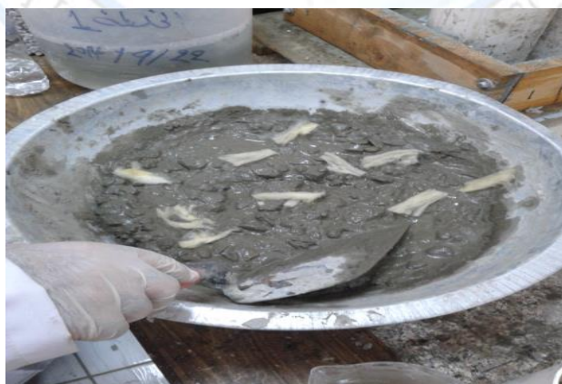
Figure (1): Mixing process of Concrete mixture and Additives.
