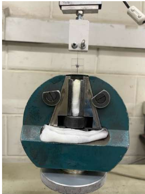
Figure 1: bracket- archwire test unit on Instron machine.
