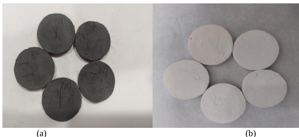
Figure 1: (a) Green body of porous ceramics, (b) porous sintered ceramics.
