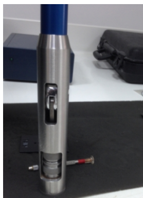
Figure (3): Hand press (Manual KBr/powder pellet press)
