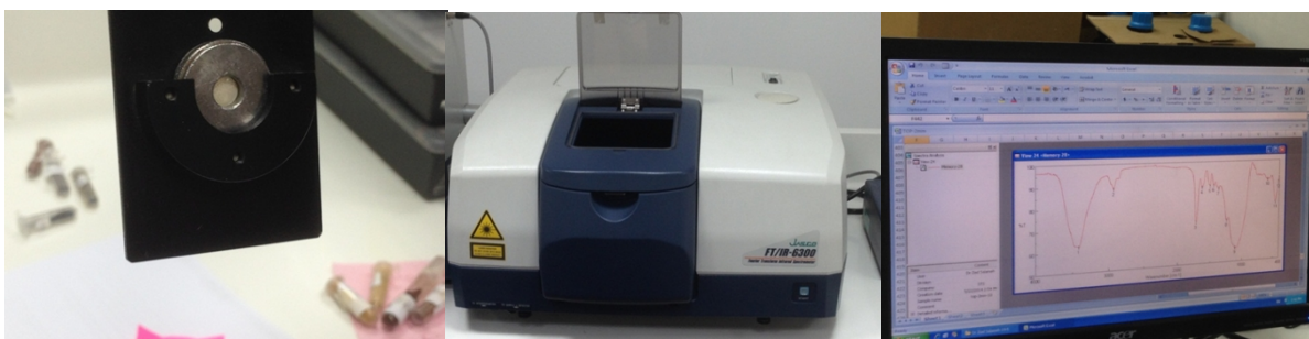
Figure (4): FTIR spectrometer (JASCO FT/IR-6300) and its spectrum after recorded
