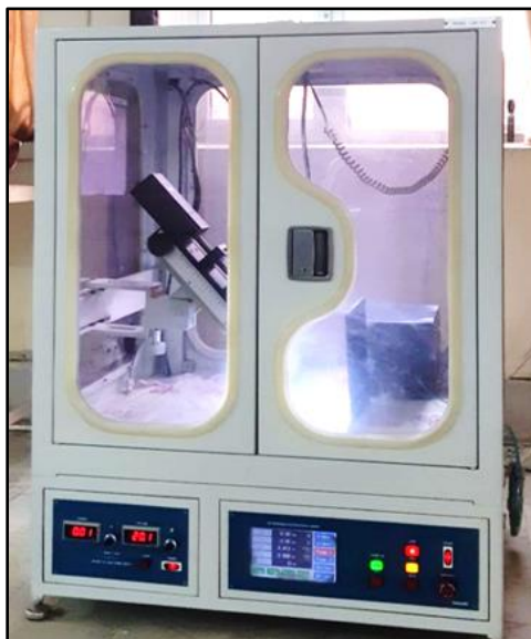
Figure 1: Photograph of electrospinning apparatus for nanofiber synthesis.
