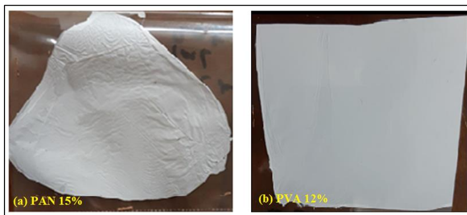
Figure 4: Photograph of the prepared air nanofilters: (a) PAN 15% and (b) PVA 12%.
