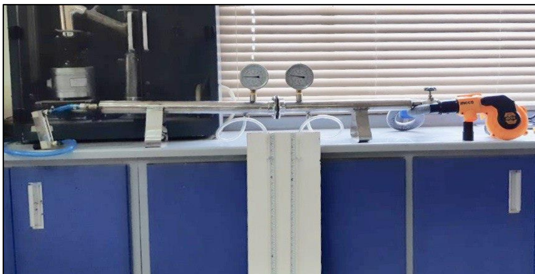
Figure 5: Photograph of the air flow system for nanofilters flow performance measurements.
