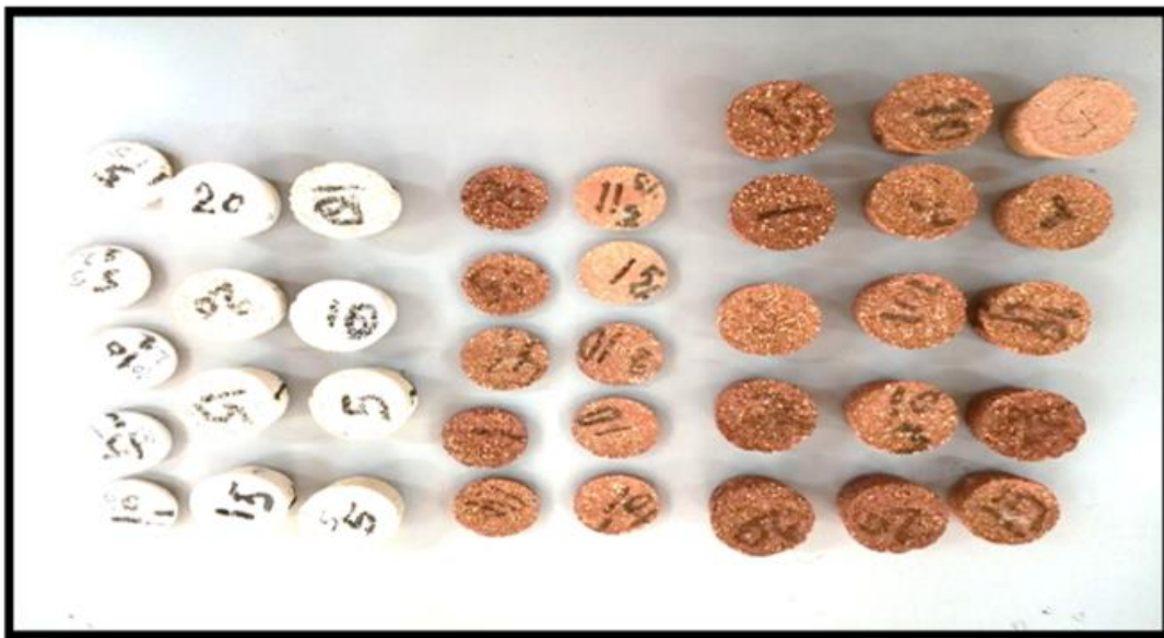
Figure 1: Specimen after firing at 1200 °C.
