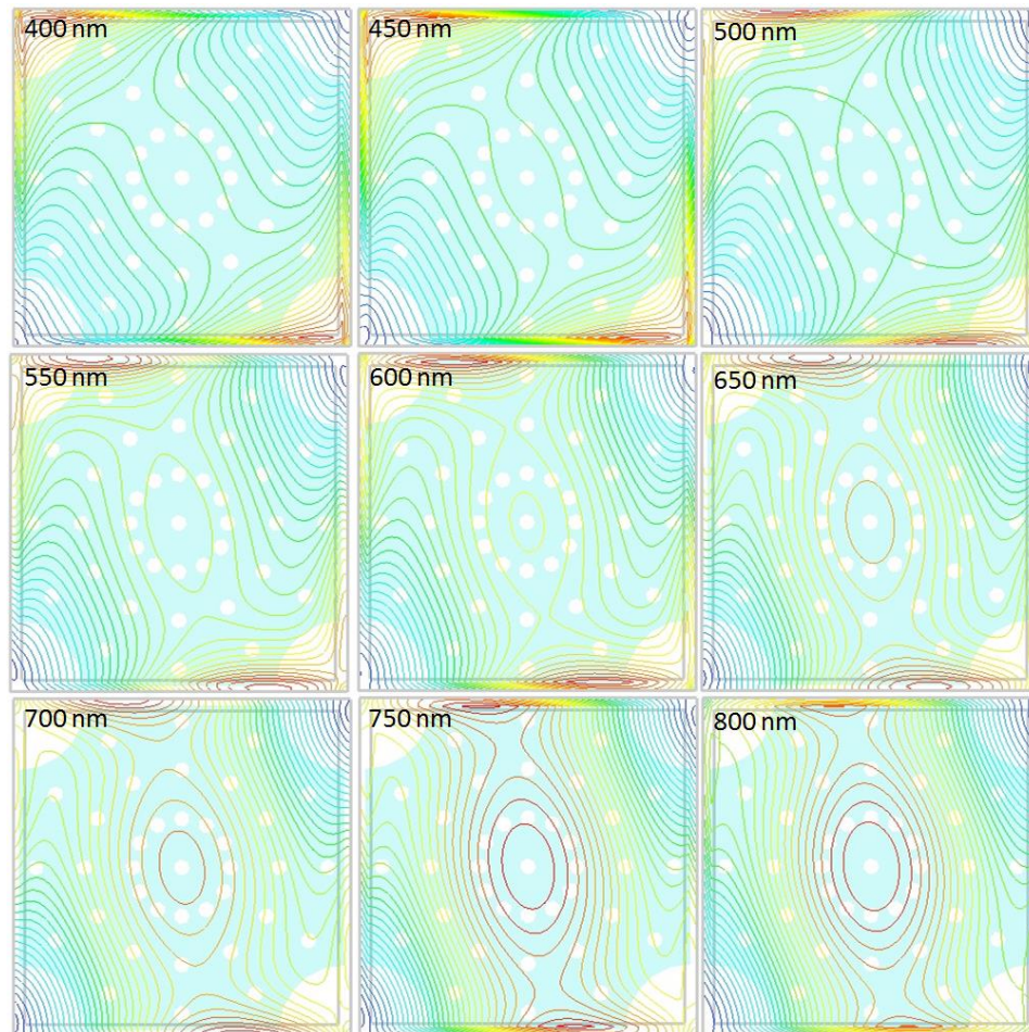
Figure 8: The electromagnetic field distributions on the surface of the proposed UC-PBG structure
