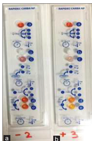
Figure 4: Representative confirmation of carbapenemase production in Pseudomonas aeruginosa isolates by using Rapidec Carba NP Test. The positivity of the reaction of tested isolate is observed in well (e) compared to the control well (d). (a) Negative result for Carbapenemase production corresponded to same color (red) as in control well, and (b) Positive result for Carbapenemase production corresponded to a color change from red to yellow
