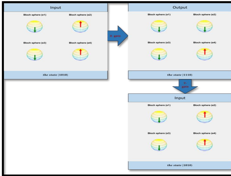
Figure 8 [the first gate (X-gate) applied on the second electron for the state |1010\rangle , after that applied (Y-gate) on the second electron for the result state |1110\rangle that change it to same state |1010\rangle ].
