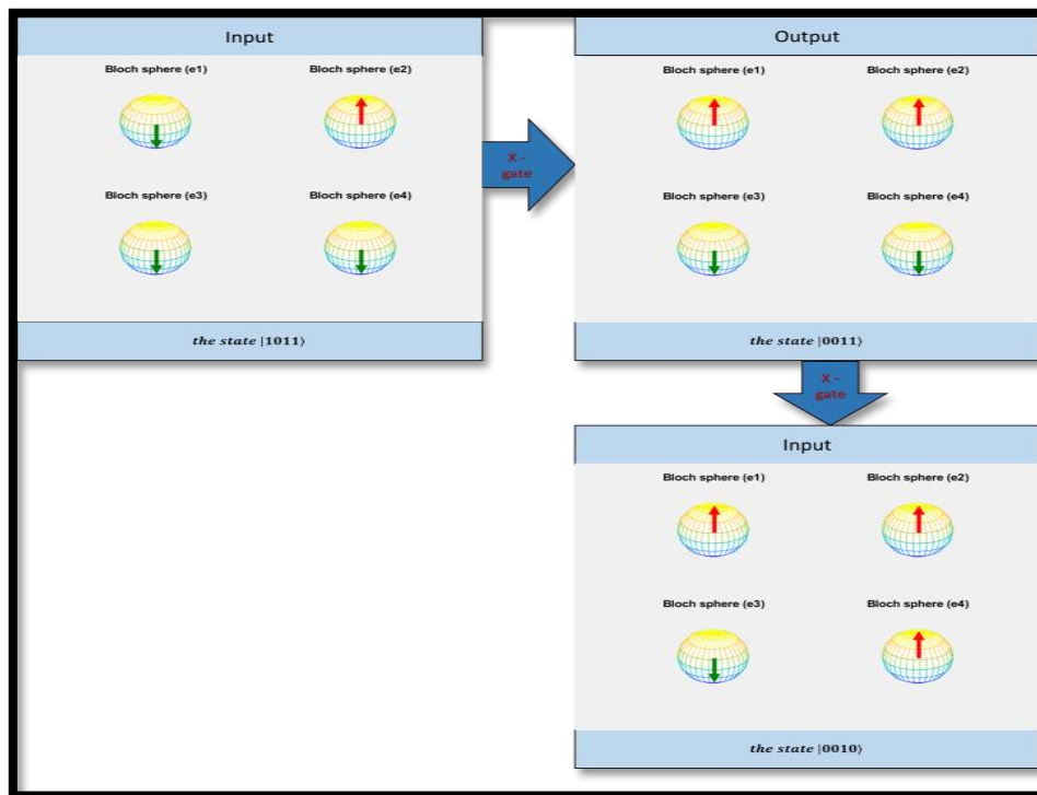
Figure 9 [the first gate (X-gate) applied on the first electron for the state |1011\rangle , after that applied (X-gate) on the fourth electron for the result state |0011\rangle that change it to state |0010\rangle ].
