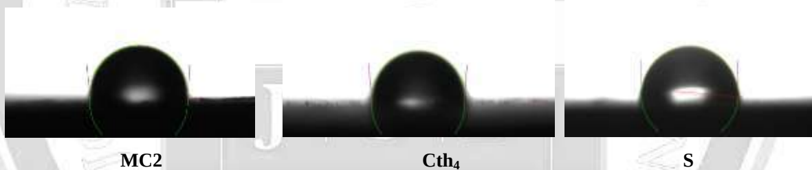
Figure 6: Contact Angle Results for Thassos Substrates.
