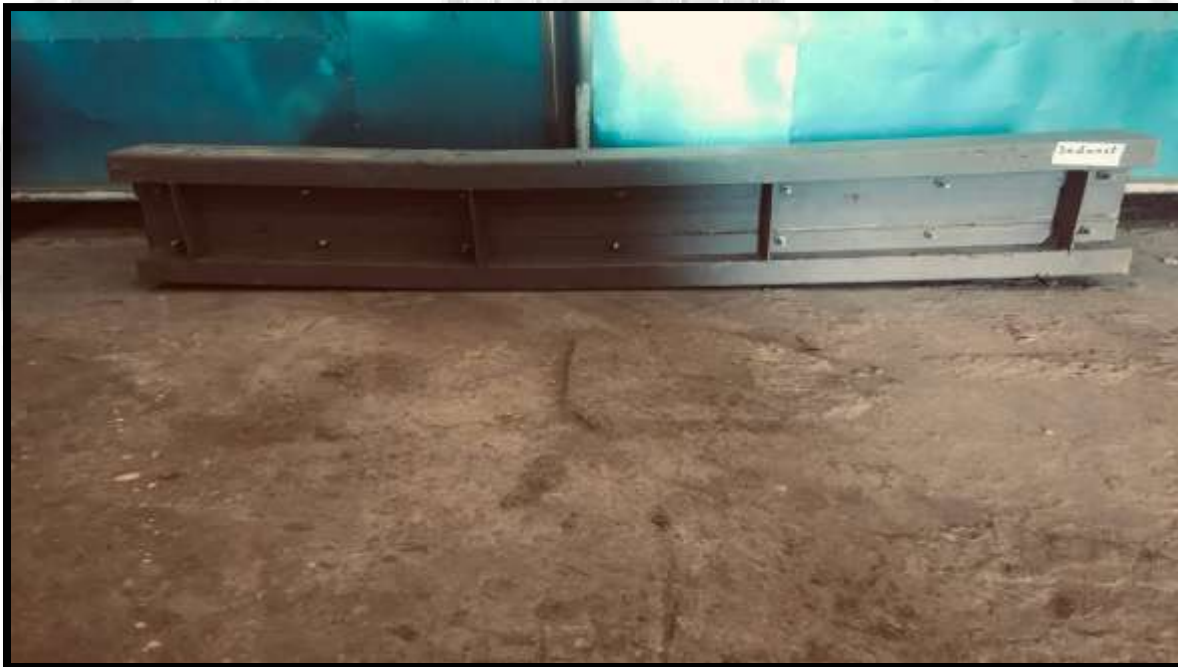
Figure (15): Failure of CFS I-beam strengthened the rectangular hollow flange by normal concrete has been replaced fine aggregate with 30% sawdust (A60S)
