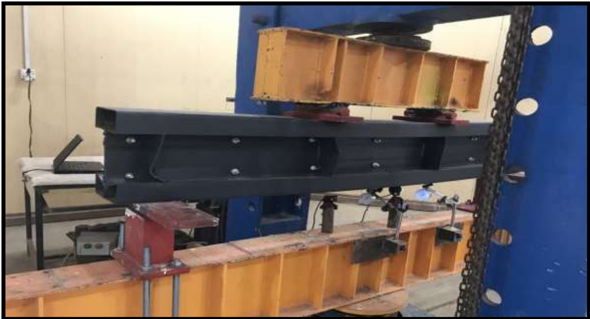
Figure (7): Failure of CFS I-beam with rectangular hollow flange (A60)
