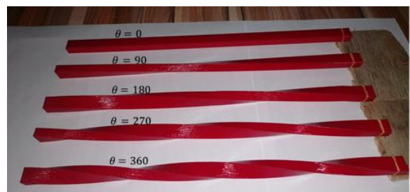
Figure 6. Beam Samples with Different Twisting Angles ( \theta ).
